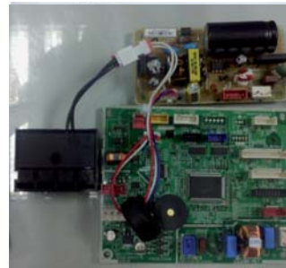
Connection of terminal block and Main PBA
